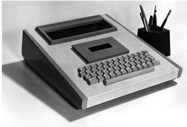
Figure 3. An early production model of the MCM/70. (Source: MCM photo, 1974.)
